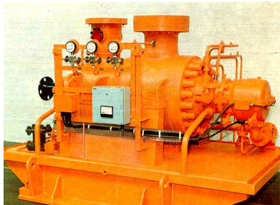
Boiler Feed Pump
